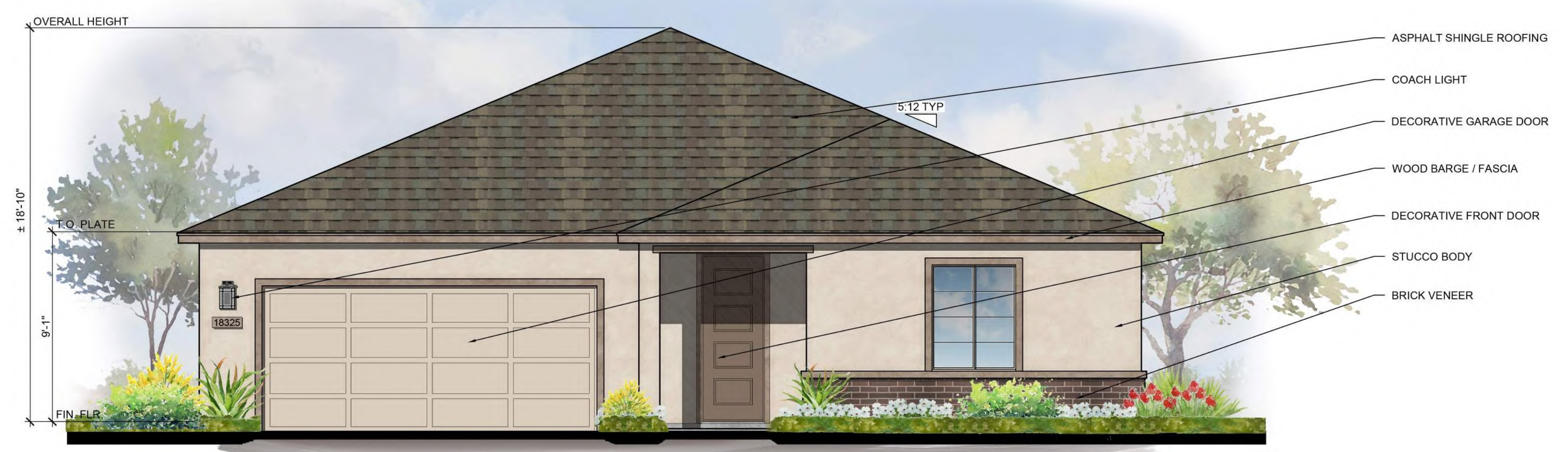
FRONT ELEVATION ELEVATION C 1/4" = 1'-0"
